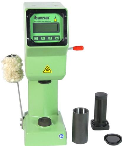
This instrument was designed to mimic the compressing action of an automatic molding machine in order to measure the effects the sand has upon its compactionabilities. Also, the device prepares standard 2" x 2" AFS or 50mm x 50mm metric sand specimens. The standard sand specimen is used in various tests including permeability, compressive strength, shear strength, etc.
